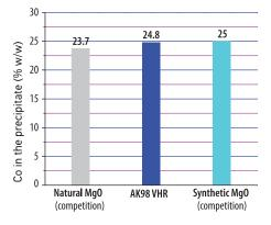
Precipitate purity using AK98 VHR and two benchmark grades. Precipitates formed with AK98 VHR exhibit higher Co concentration compared to the natural MgO and equivalent to that obtained with the synthetic MgO.
