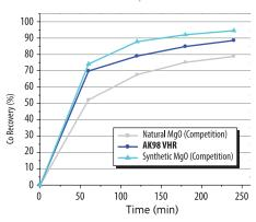
Cobalt Recovery using AK98 VHR and two benchmark MgO grades. AK98 VHR achieves higher recovery than the natural MgO and closely follows the recovery achieved with higher priced synthetic MgO.
