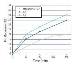
Nickel Recovery (left) and corresponding Manganese recovery (right) using AK98 VHR at various MgO/(Ni+Co) ratios. AK98 VHR exhibits high selectivity at low MgO loadings. In this example, Ni recovery after 3 hours and at only 2% above stoichiometry (i.e. MgO/(Ni+Co) = 0.7), is almost 94% while the corresponding Mn impurity recovery is less than 20%. Higher ratios can increase Ni recovery up to more than 99% but with Mn recovery reaching higher levels.
